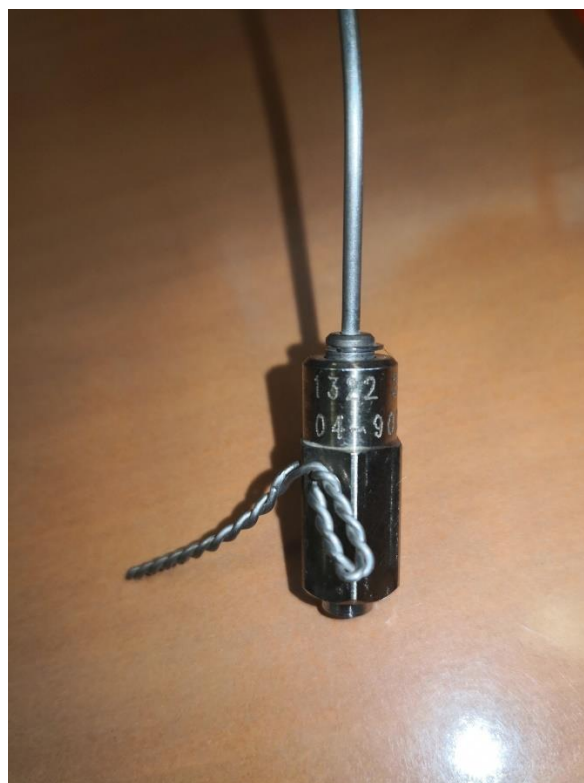
Figure 4-51. Identification Markings on Coaxial SE Female (Socket) Connector
