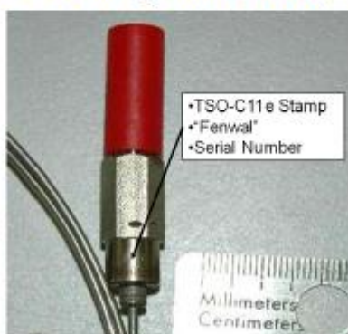
Figure 4-51. Identification Markings on Coaxial SE Female (Socket) Connector
